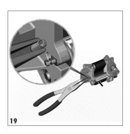
• Press the pinch roller against the transport belt and hook the spring.
