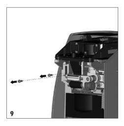
• Remove the socket-head screws from belt drive with the SW 2.5 Allen key.
