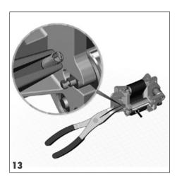
• Unhook the spring with an bent long nose pliers.
