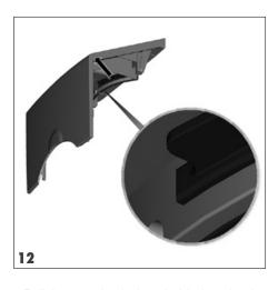
• Pull the guard strip from behind so that it slips through the slots.
