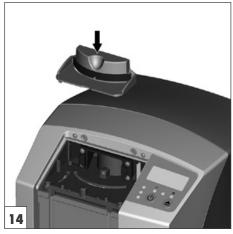
• Insert the retaining plate.
