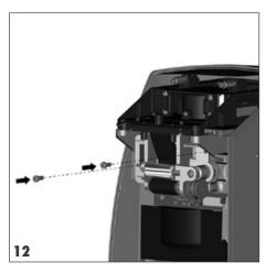
• Fix the belt drive in place using two socket-head screws and the SW 2.5 Allen key.
